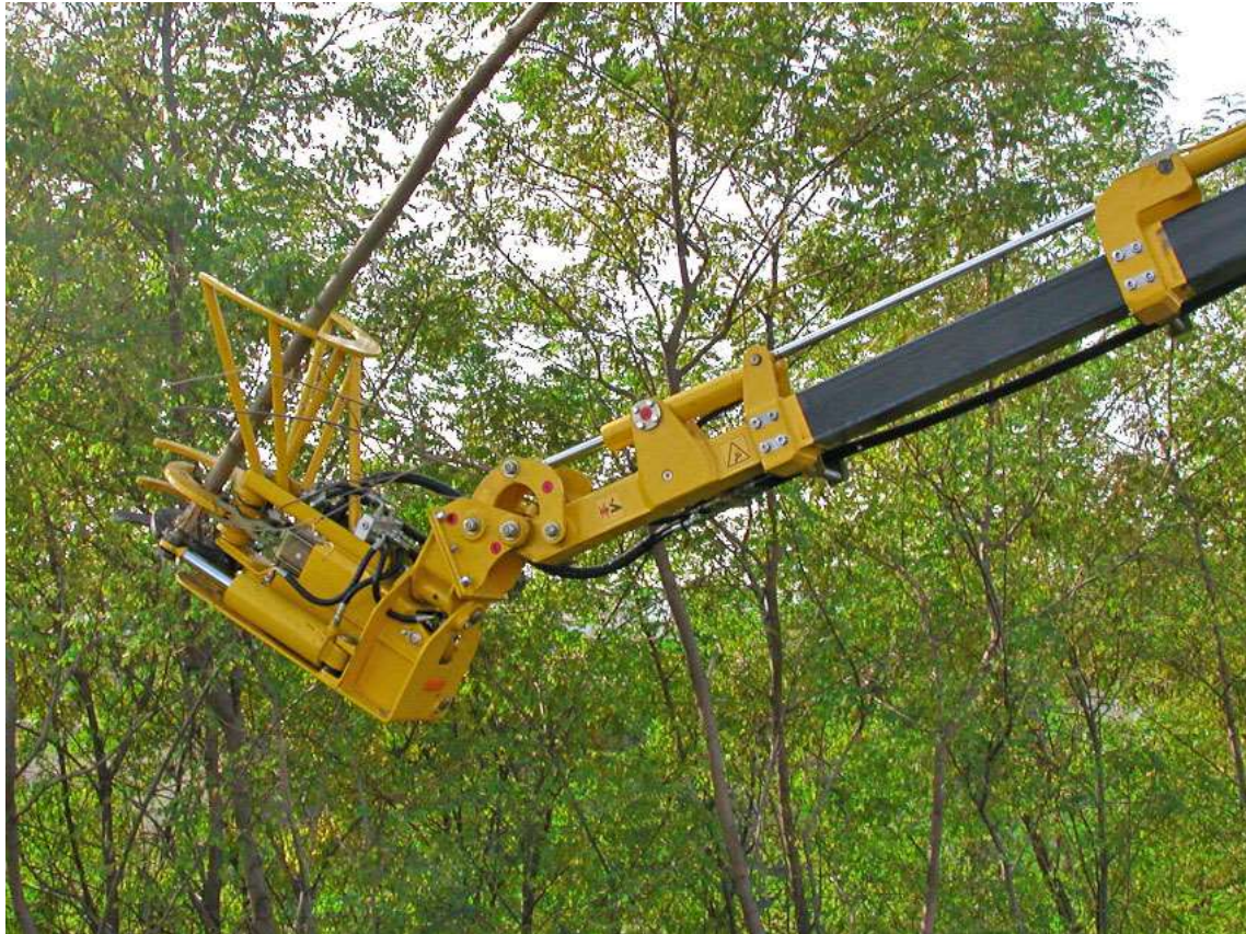
Figure 4: Proven wood harvesting technology: Hydraulic pruning scissors with long reach. (Source: Energreen Italy).
