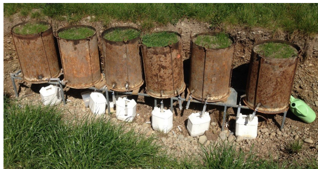
Figure 2 Research lysimeters Pastoral 21 research trial Ashley Dene near Lincoln
