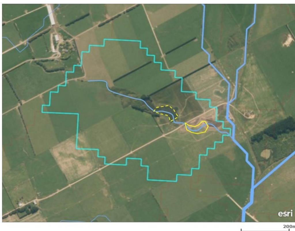
Figure 1: Location of Warnock's Farm wetland and phosphorus filters. The catchment boundary has been generated in ARC GIS (ESRI). The boundary of this catchment is outlined in teal. Flow paths have been shown with a light blue line. The constructed wetland location is outlined by a solid yellow line (satellite imagery taken before wetland construction). The duck pond is outlined in a dashed yellow line.
