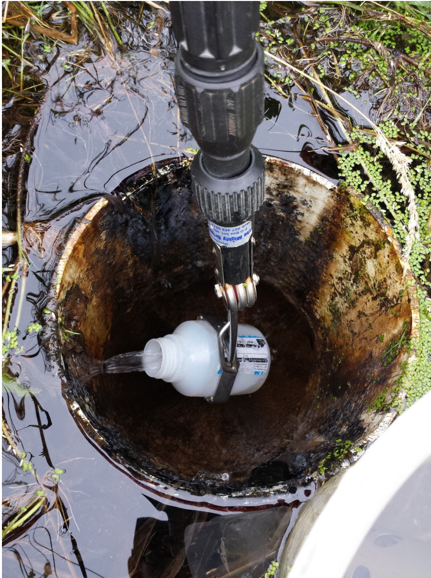
Figure 8: Sample collection from one of the outlets. (Credit: Aquatech/Environment Southland).
