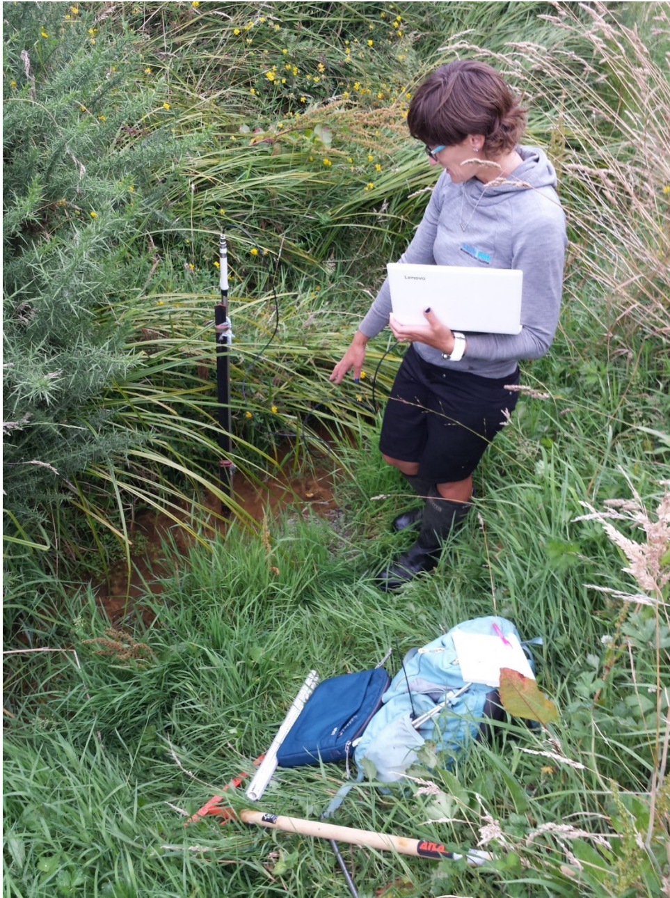
Figure 9: Water depth monitoring location. Dianne Elliott, Aquatech. (Credit: Aquatech/Environment Southland). Note iron floc in the water.
