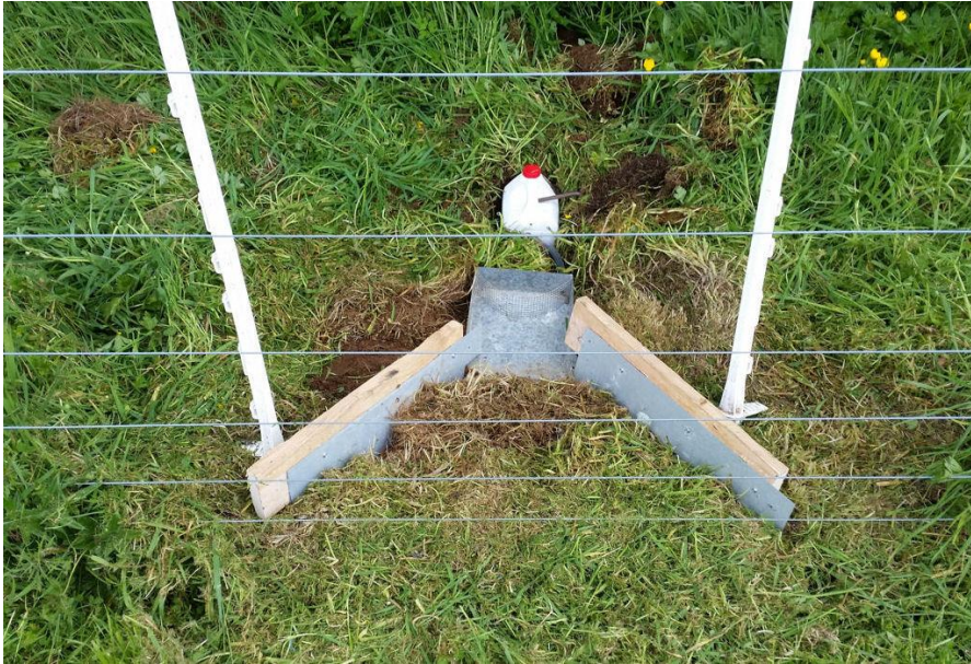
Figure 2. Run-off collector at Butterworth farm
