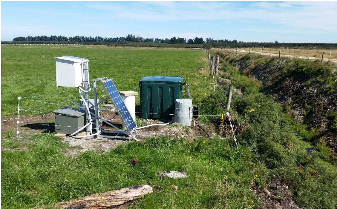
Figure 2-4: Photographs of P filter showing key components of the monitoring equipment at the as-built filter.
