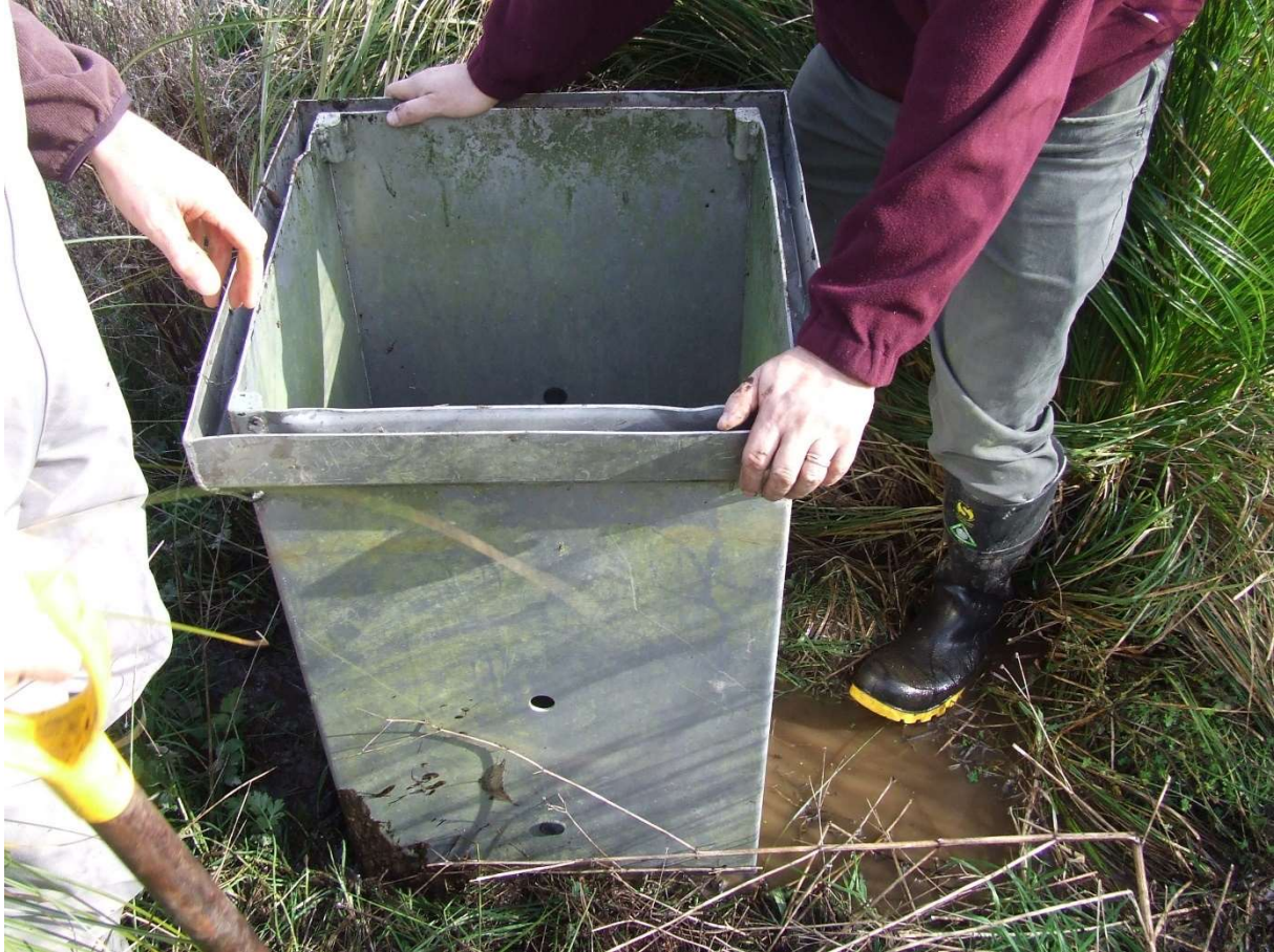
Figure 4: Mesocosm being installed in a seepage wetland.
