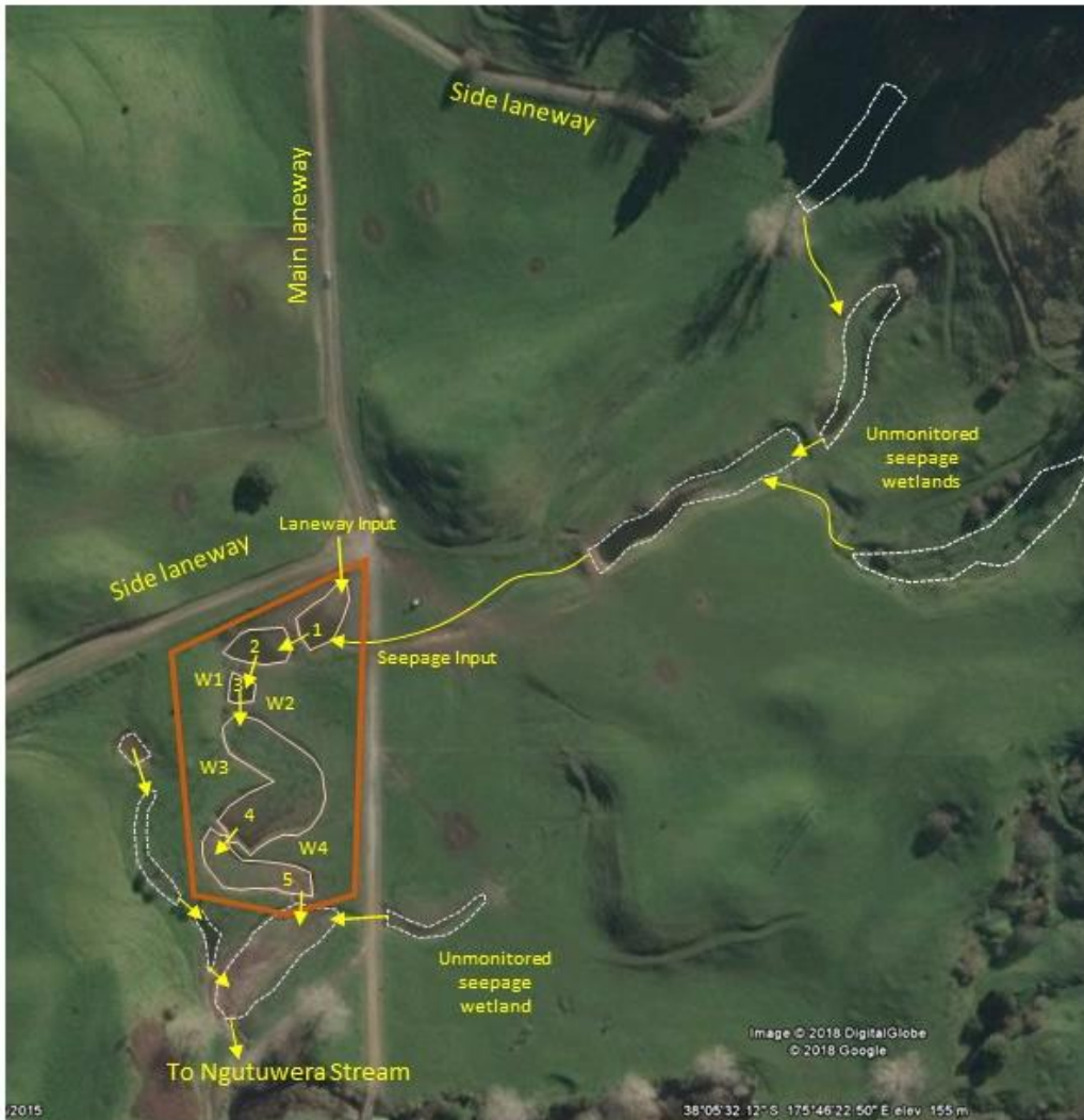
Figure 1: Layout of constructed wetland along with major inlets and outlets. The five monitored constructed wetland cells are defined with pink unbroken lines and have been enclosed within an orange boundary. Unmonitored wetland cells (constructed and natural seepage) are outlined in broken white lines. Laneways that contribute to the laneway input are identified. W1-W4 are the groundwater sampling wells.
