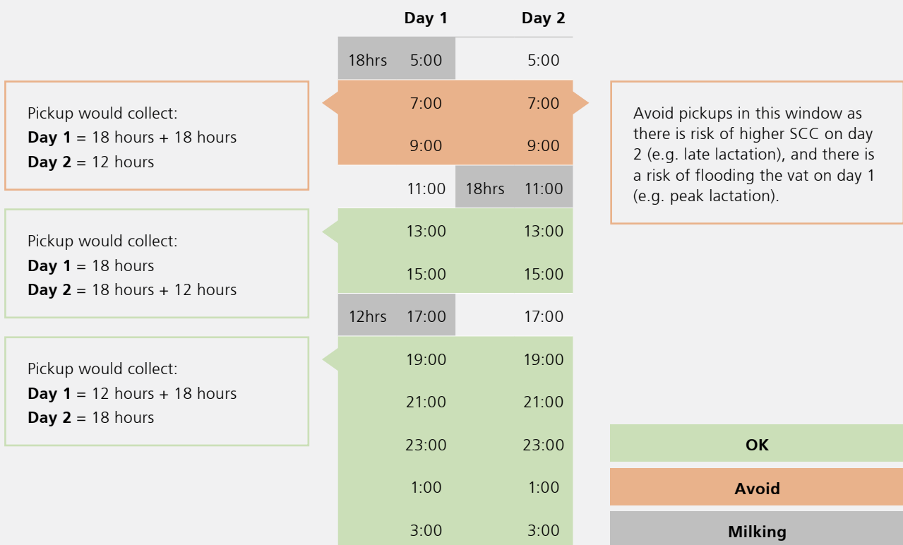
Figure 4. Tanker scheduling options assuming a daily pickup and the tanker coming in the same window each day
