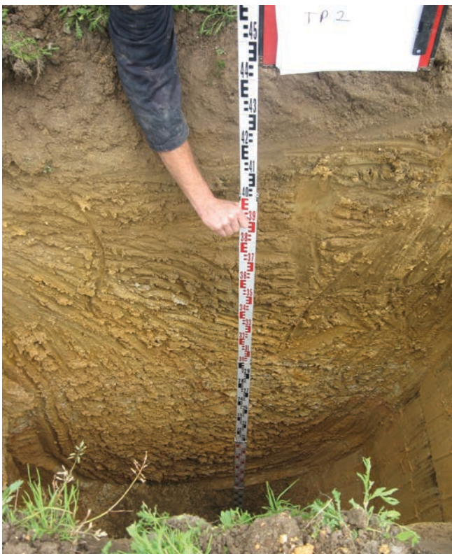
Investigation trial pit
