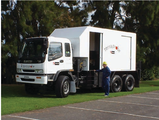
Figure 4.1: Truck and Track-Mounted CPT Vehicles
