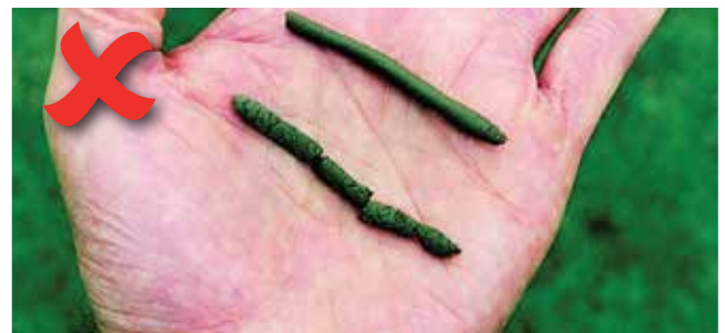
The soil makes a 'worm' when rolled, sticks to your thumb when rolled or free water appears when squeezed.
